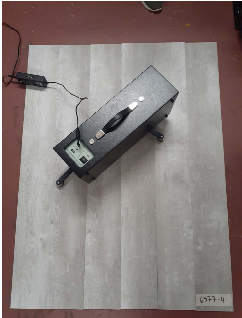
Figure 2. Image of test configuration - 'ID Comfort 19' laid on top of base floor
